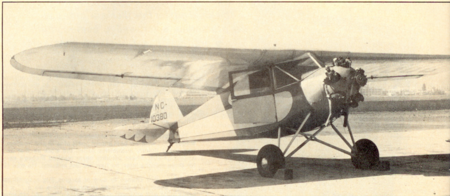
The 90-hp, type-certificated version of the Kari-Keen Coupe, built in 1930. Note the rigid round-tube landing gear; all shock absorbing was by the Musselmann-designed Goodyear "Airwheels." Photo by Gordon S. Williams.
